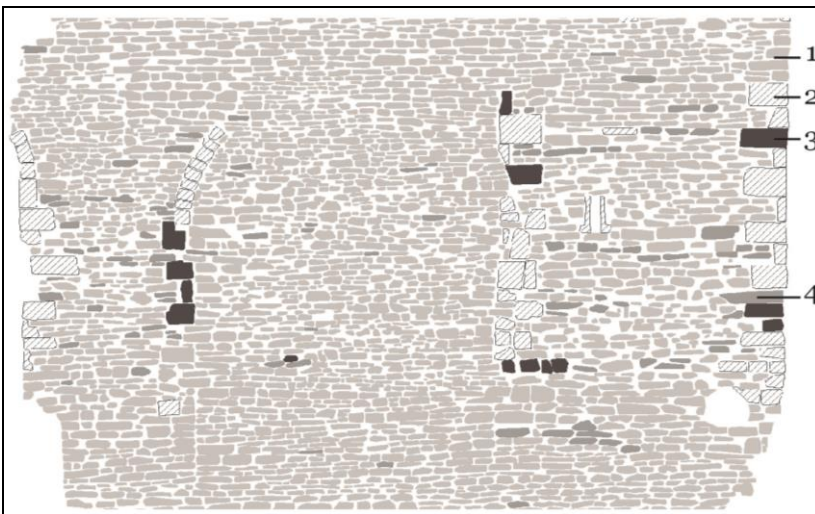
Figure 3. Example of a lithological map (width 10 m) showing the northern façade of the Cathedral of Santa María, 1. Campanian calcarenite ( Calcarenitas de Olárizu ); 2. Paleocene limestone ( Lumaquelas de Ajarte ); 3. Paleocene dolomite; and 4. Campanian marly limestone of the substrate (Image of the Fundación Catedral Santa María)
