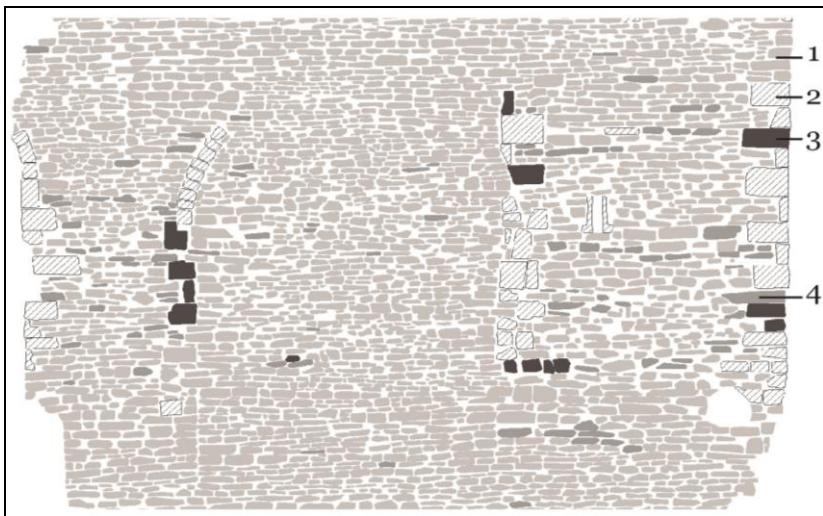
Figure 3. Example of a lithological map (width 10 m) showing the northern façade of the Cathedral of Santa Maria, 1. Campanian calcarenite ( Calcarenitas de Olárizu ); 2. Paleocene limestone ( Lumaquelas de Ajarte ); 3. Paleocene dolomite; and 4. Campanian marly limestone of the substrate (Image of the Fundación Catedral Santa María)
