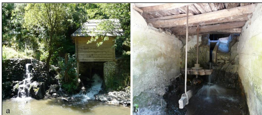
Figure 3. Watermill on Rudăria valley (a); Functioning mechanism of a watermill (watermill wheel - "ciutura") (b)
