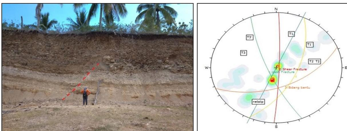
Figure 8. An outcrop showing the Apitalawu Fault (left) and fault data processing results (right)
