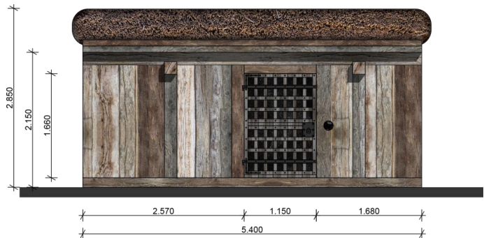
Figure 12. Façade of wooden, mud brick and reed cellar, Salacea
