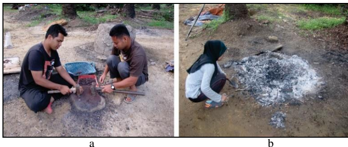
Figure 9. The process of breaking iron ore into small lumps (a) and the roasting process (b) (Source: Research data analysis, 2023)
