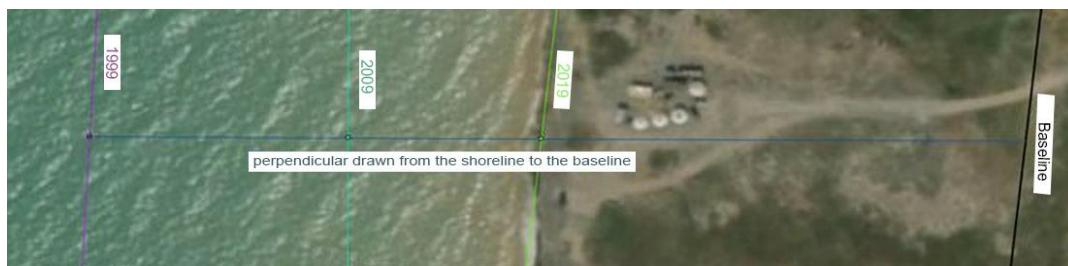
Figure 5. Interrelationship of NSM, EPR, SCE indicators, NSM = distance between oldest and latest shoreline (m), SCE= distance between two extreme shorelines (m)
