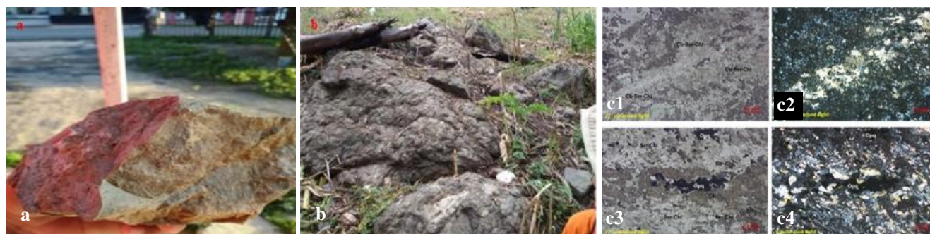
Figure 4. (a) Hand specimen of andesite lava in Karya Murni Village (b) Pillow lava structure on andesite outcrop in Karya Murni Village, (c) Photomicrograph of andesite rocks. Photomicrograph shows the minerals found in andesite rocks. The photomicrograph on the left uses polarized light (c1 and c3) while the photomicrograph on the right uses x-polarised light (c2 and c4). The minerals visible in the photomicrograph are plagioclase, orthoclase, and pyroxene (Source: Field documentation and research data analysis, 2019)
