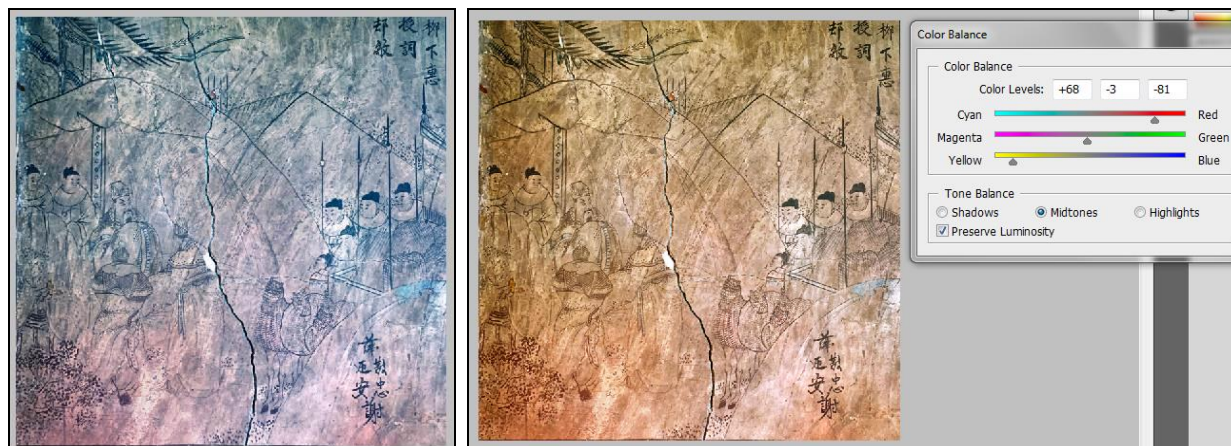
Figure 9. Color-balancing procedures for natural color
