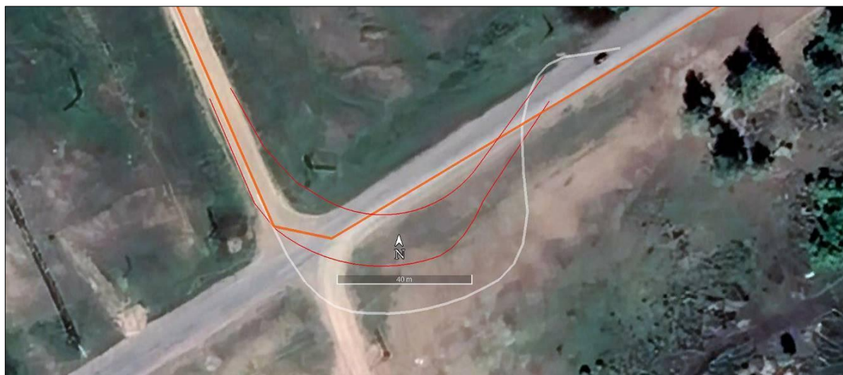
Figure 5. The blades transporting trailers right-angle turn after Osakarovka (brown line) allows for the blades (white line trajectory) to avoid the powerline poles but will require ground enforcement for driving outside the road (red lines trajectory). (Source: Base map source: Google Maps, 2025. Annotations and layout by the authors)
